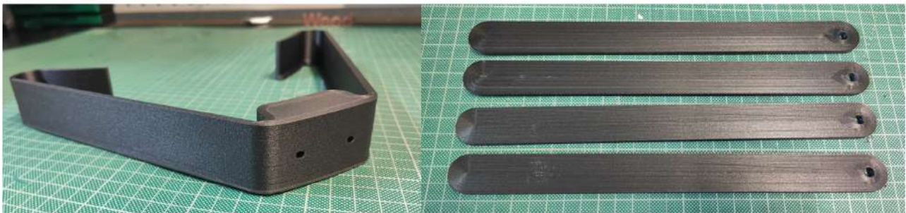
Figure 9. Example of precision components manufactured at AIMEN using PC-CF composite filament from 3DXTECH® [3].
