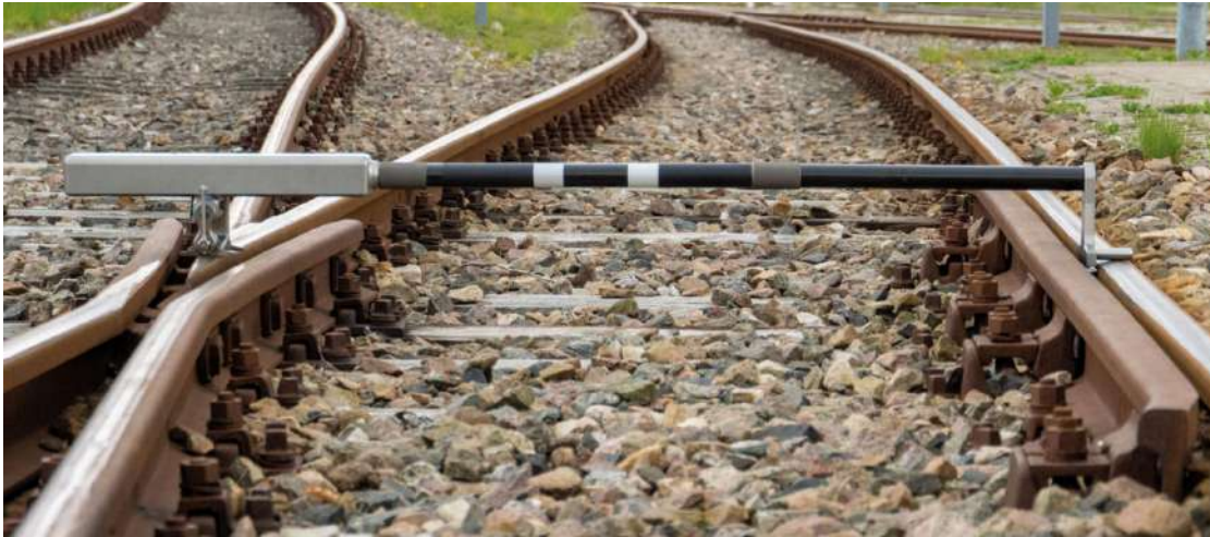
Figure 6. MiniProf [1] profile wear assessment device inspecting wear at nose section.
