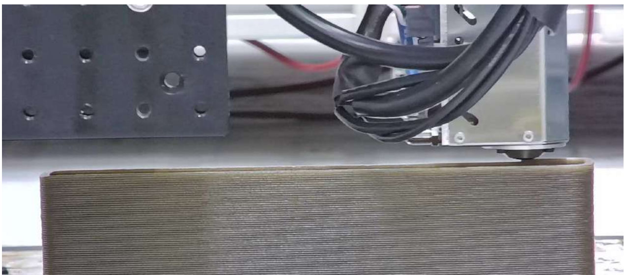
Figure 14. Manufacturing process using Typhoon [6] FFF printhead.
