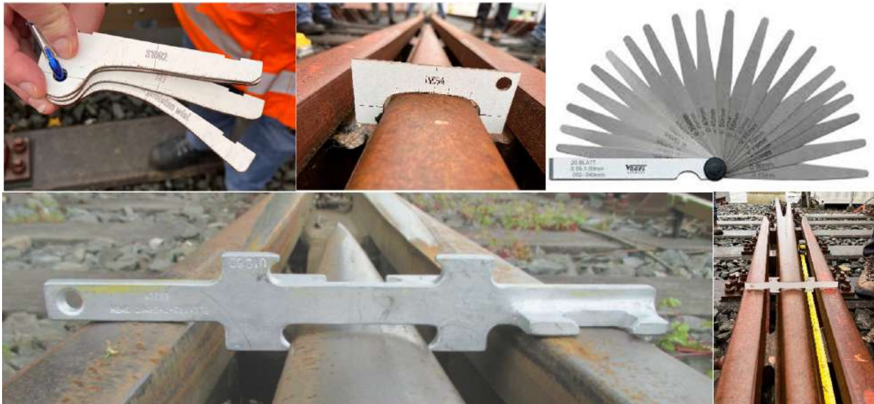
Figure 2. Current manual gauges and templates used for manual verification of manual repair works. Image courtesy of ProRail and RET.
