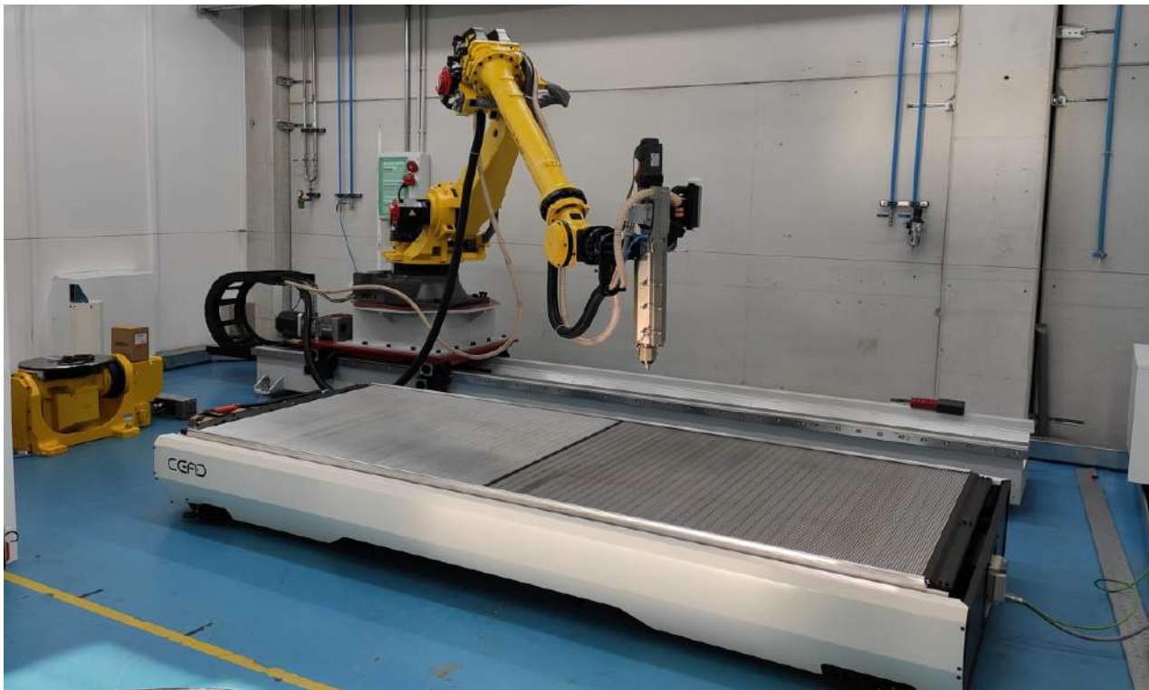
Figure 10. LFAM robot cell with FGF equipment from CEAD B.V [5].
