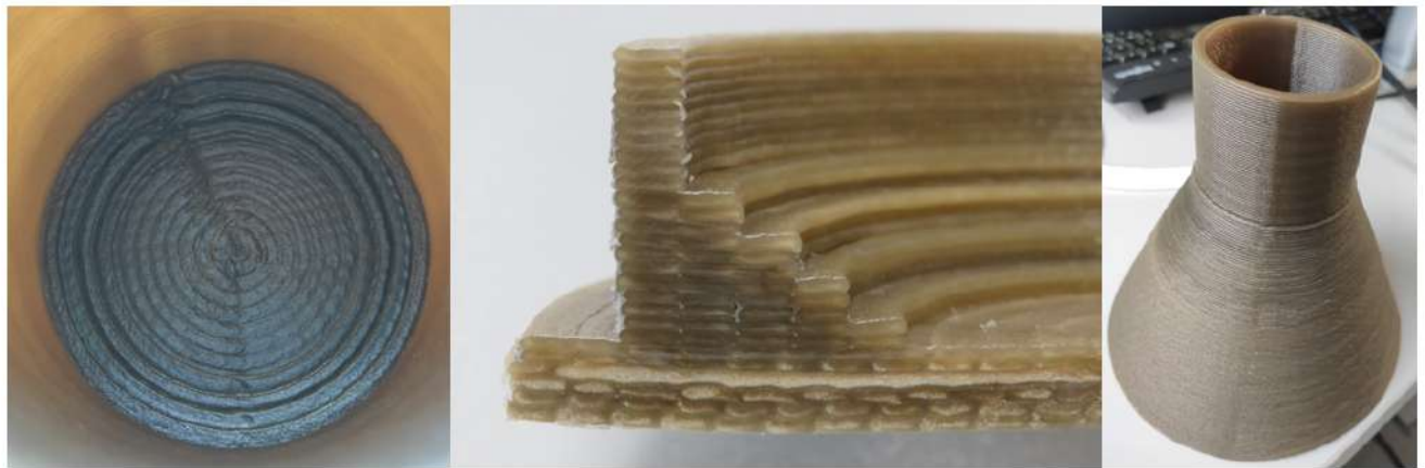
Figure 15. Example of medium format parts manufactured with FFF Typhoon printhead at AIMEN using PA composite material. Central image displays cross section to appreciate resolution of printed layers of 1mm height.
